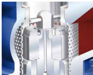
Flow divider for noise reduction
