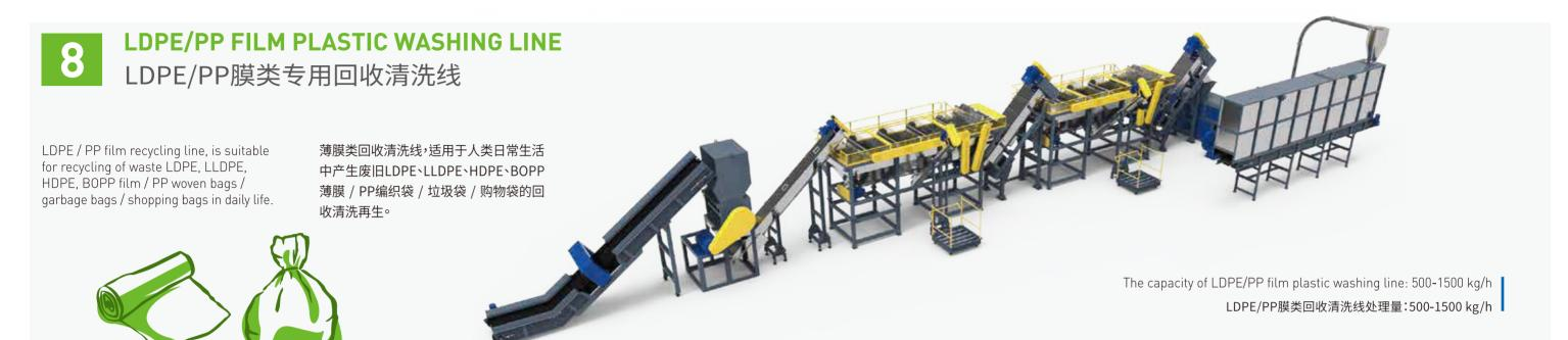
The 3D flow chart is a general process flow, it will be designed according to the raw material condition and the customer demand. 3D流程图仅为一般工艺流程示意,实际依据原料状况及实际厂况排布
