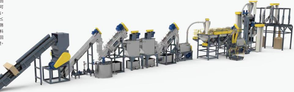
The capacity of PE Motor Oil Container Recycling Line: 500-1000 kg/h
