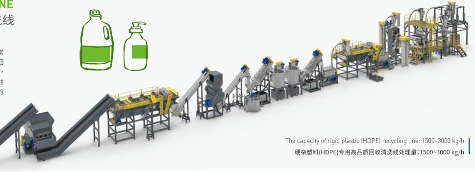
The 3D flow chart is a general process flow, it will be designed according to the raw material condition and the customer demand. 3D流程图仅为一般工艺流程示意,实际依据原料状况及实际厂况排布
