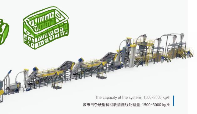
he 3D flow chart is a general process flow, it will be designed according to the raw material condition and the customer demand. 3D流程图仅为一般工艺流程示意,实际依据原料状况及实际厂况排布
