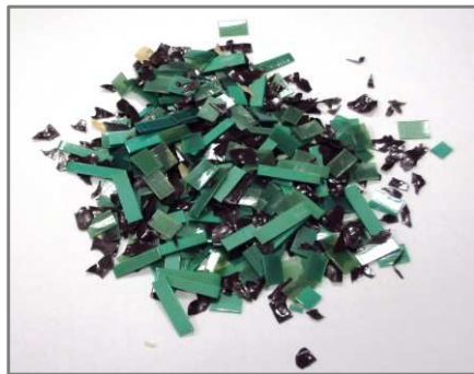
Regrind of strap and thermoforming sheet in PET
