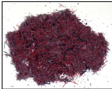
Regrind of monofilament for brooms in PET+PE/PP
