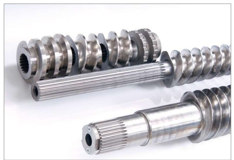
분할형 스크류(segments): intake, mixing elements, discharge
